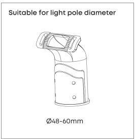
If the fixture is installed by post top, please release the screws on the bracket behind the fixture and remove the bracket first, then turn the bracket in the opposite direction, use a 6# hex wrench to tighten the screws to fix the bracket, as shown below.
