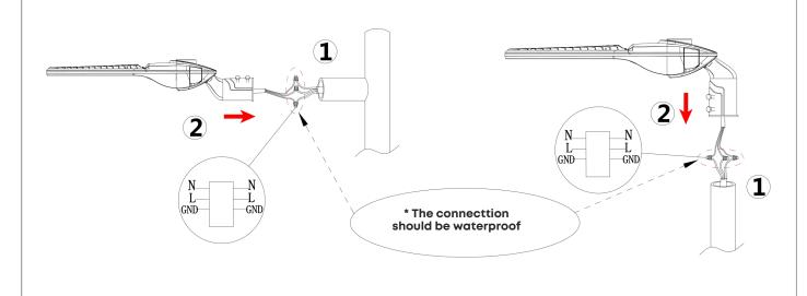
3. Tighten the two screws.
