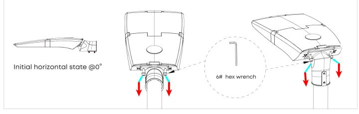
5. Rotate the fixture to the proper angle based on the actual requirement, then tighten two screws behind the fixture on the bracket.
