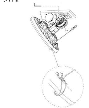
Step 10: Insert the elbow of the lamp into the lamp post and tighten 4 fixing screws with an inner hexagon wrench. The torsion:19-22 N\*m.
