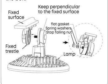
Step 8: Tighten the fixing screw with an inner hexagon wrench. The torsion:13-17 N\*m.
