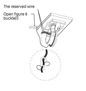
Step 5:Put the power cord out of the bracket, then fix the rotating bracket on the lamp body,tighten the screw.
