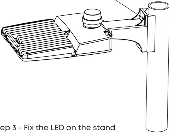
Step 3 - Fix the LED on the stand adapter and secure with the M8 screw
