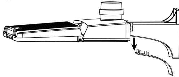
Step 2 - Remove the screw and open the cover
