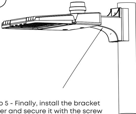
Step 5 - Finally, install the bracket cover and secure it with the screw
