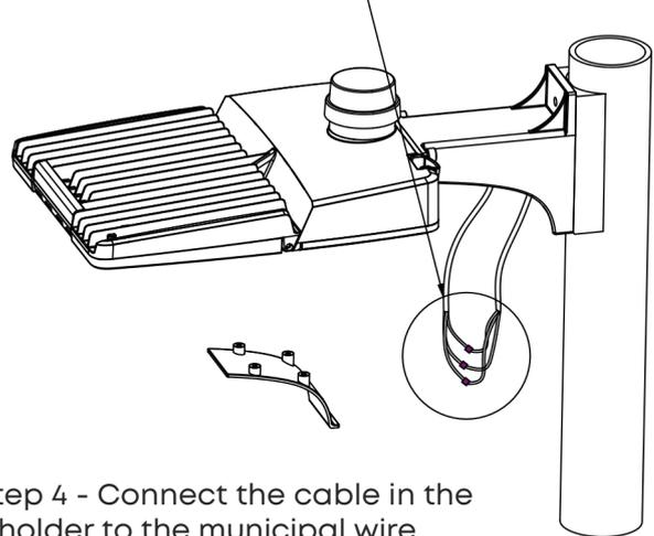
Step 4 - Connect the cable in the F holder to the municipal wire, as shown in Figure F or G
