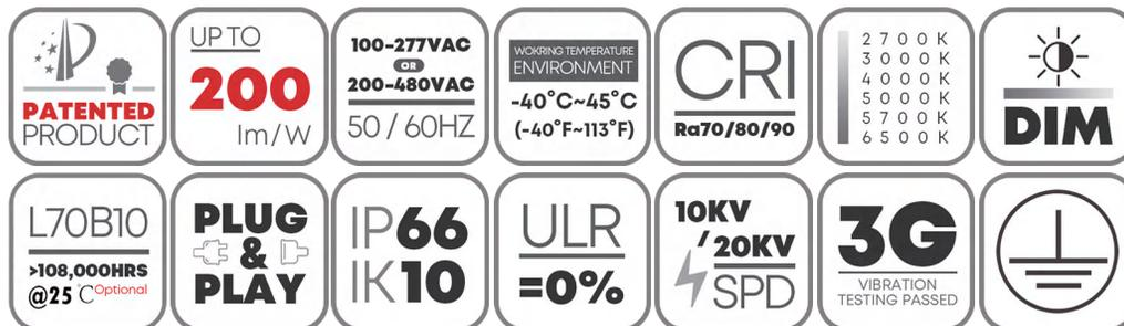
Note: Normal Voltage=100-277VAC, High Voltage=277-480VAC, please evaluate before choosing. For the power supply in the United States and Canada, in case the input voltage fluctuation  $\geq 240V$  the High Voltage solution is highly recommended for performance stability. Improper selection will cause damage to the driver or the light.
