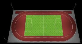
Reference Data Field proportion: 105\*68m; Installation height: 50m; Pole number: 4 PCS; Number of fixtures: 5 PCS \*4; The total lumens: 144000lm; Power of each fixture: 1200w;
