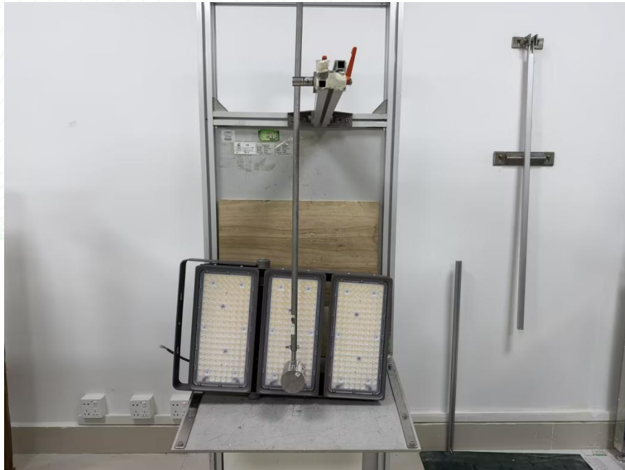
Photo 3: IK08 test of model AOK-600WFLD-NV-L2-6570-30D-T
