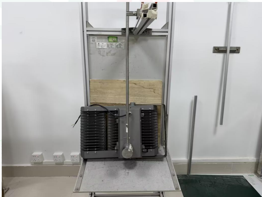
Photo 4: IK08 test of model AOK-600WFLD-NV-L2-6570-30D-T
