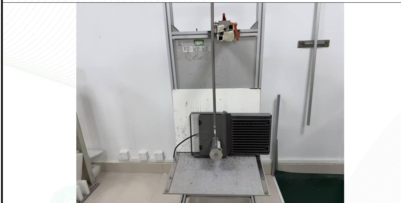
Photo 5: IK09 test of model AOK-200WFLC-NV-S5-00-6570-60-P
