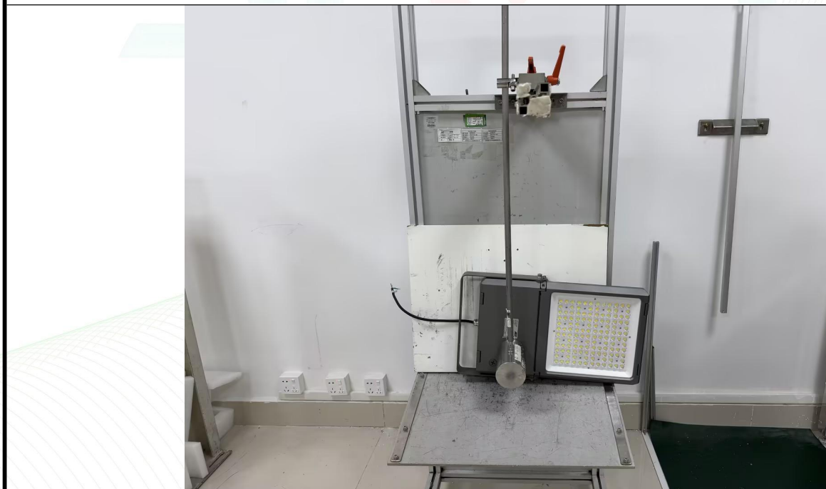
Photo 4: IK09 test of model AOK-200WFLC-NV-S5-00-6570-60-P
