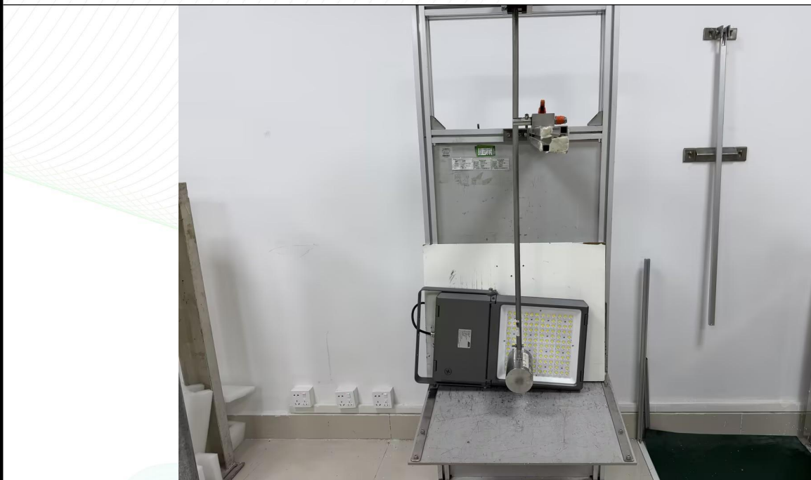
Photo 3: IK09 test of model AOK-200WFLC-NV-S5-00-6570-60-P
