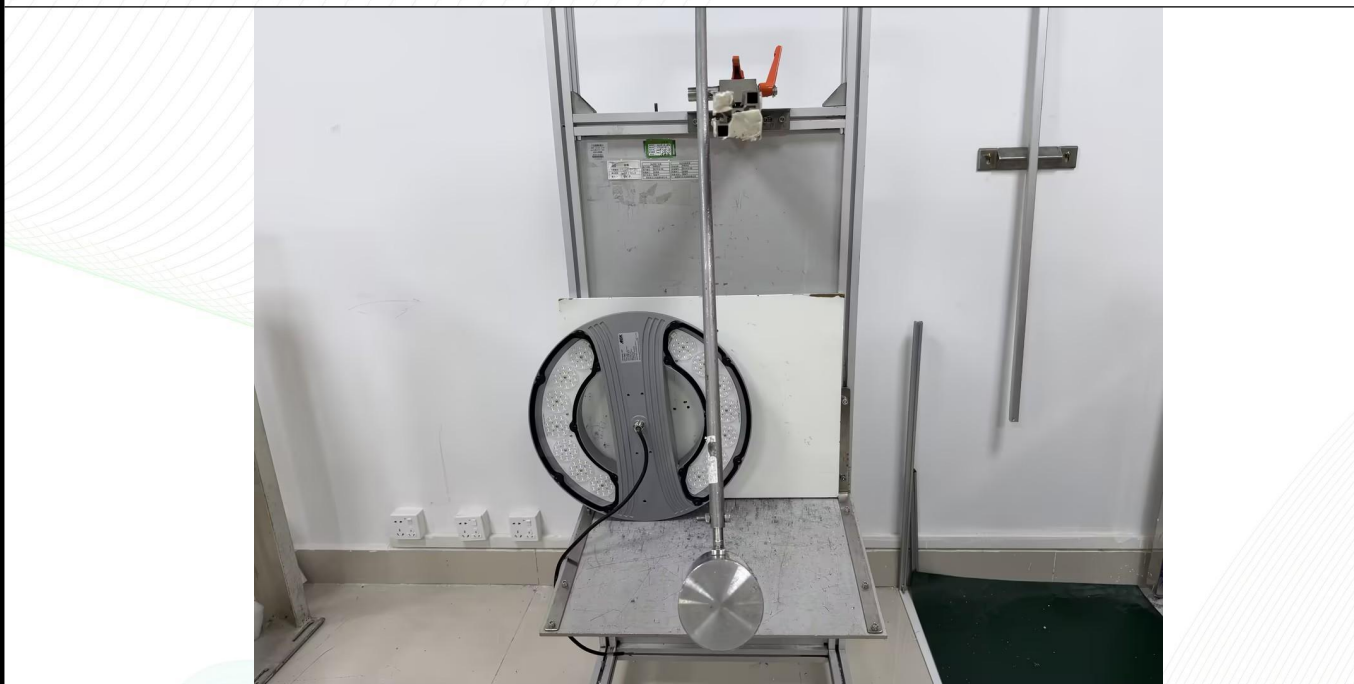
Photo 3: IK09 test of model AOK-120WIP-NV-L2-00-6570-T4-P
