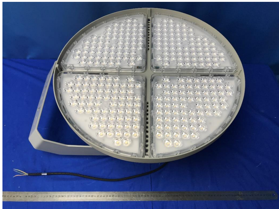
Front panel view of AOK-960WiNS-NV-XX-XX-XXYY-BN-P after 1000 hours salt spray
