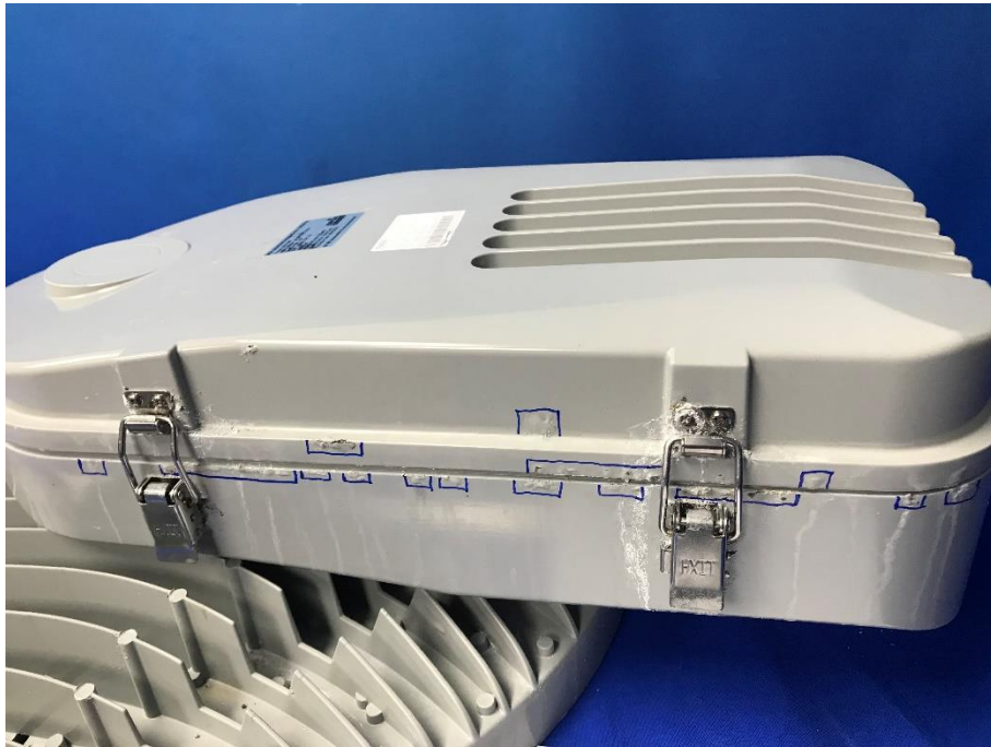
Detailed view of AOK-580WiNM-NV-XX-XX-XXYY-BN-P after 1000 hours salt spray
