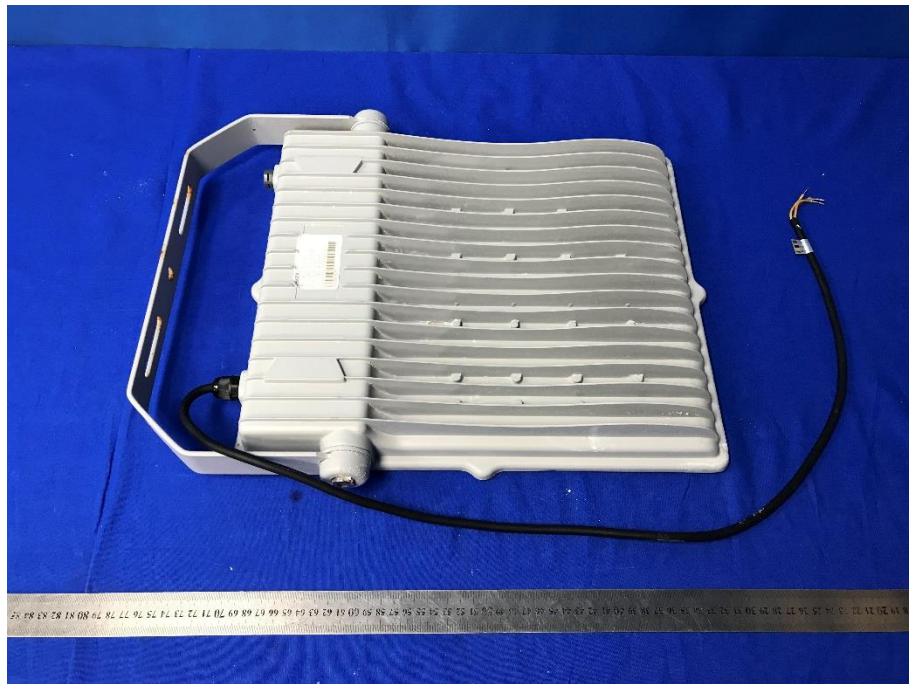
Rear view of AOK-230WiF-NV-XX-XX-XXYY-BN-P after 1000 hours salt spray
