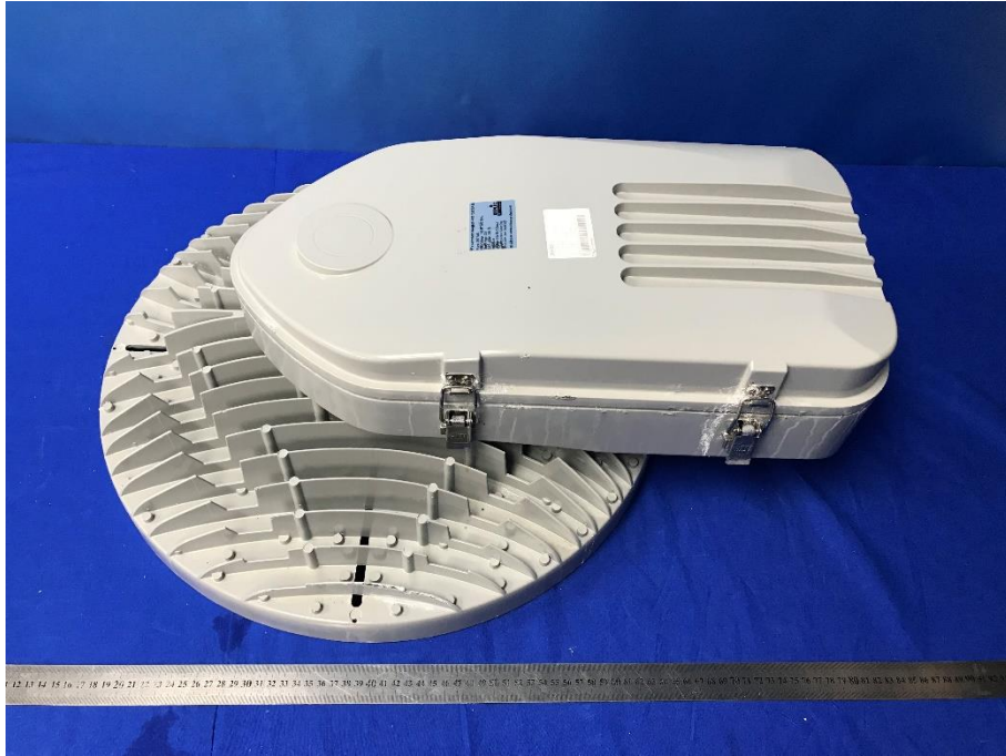
Overall view of AOK-580WiNM-NV-XX-XX-XXYY-BN-P after 1000 hours salt spray
